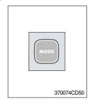
(1) Operating this switch, it beeps and displays symbol of each mode in order.(Vent  $\rightarrow$  B/L  $\rightarrow$  Foot  $\rightarrow$  Def  $\rightarrow$  Vent)
