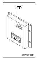
(1) Three LED lamps on the MCU controller display as below.
