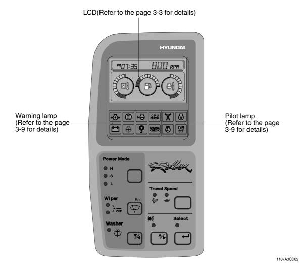
\* The warning lamp lights ON and the buzzer sounds when the machine has a problem.
